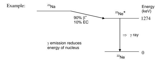
Gamma-ray energies  $E_{\gamma}$  typically, are in the range 0.1 to 10 MeV and can be determined very accurately with a modern detector.  $E_{\gamma}$  is characteristic of the emitting nucleus and are widely used to identify radioactive nuclei.
