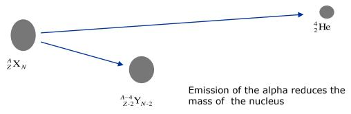
The parent nucleus  ${}^{A}_{Z}X_{N}$  emits an  $\alpha$  particle. The daughter product is 4 mass units lighter and with 2 fewer units of electric charge:  ${}^{A-4}_{Z-2}X_{N-2}$ .
